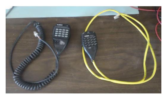
I had previously used some yellow Cat 5 network cable. Seems now a few years later, the jacket of the cable has gotten quite stiff. During the original rework, I was also not too happy with the flexibility of the individual stranded conductors and insulation.
