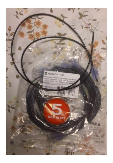
I chose the first and thinner of the two cables for the first assembly. Cut the cable in half and ended up with a 38 inch finished length. The conductors are 30 AWG, and very flexible, so as not to stress the microphone's internal circuit board solder pads.
