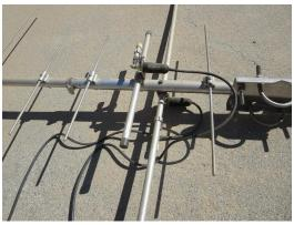
This antenna, still being produced by Cushcraft that retails for \$210 new offers a combined VHF/UHF antenna in one package. Both the VHF and UHF sections individually feature 5 element Yagis for each band. The T-coupler shown can be connected to a transceiver that outputs both a VHF and UHF signal on the same antenna port, or, alternately, separate coaxes can be connected to each antenna separately. Works great with a TV-type antenna rotor.
