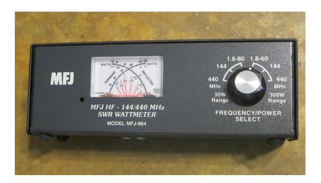
This MFJ-864 Wattmeter, still being produced by MFJ that retails for \$140 new can measure both forward and reflected power from 1.8 to 60 MHz using two power ranges, 30W and 300W. The frequency covers all the typical HF, VHF and UHF amateur frequencies which makes it perfect for any transmitter capable of up to 300 Watts output.
