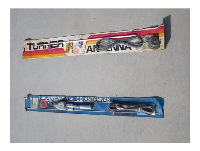
These 11-meter CB magnetic mounted car antennas were originally purchased to be modified for 10-meter operation by shortening the antenna length. Obviously, this was never done but it otherwise provides a great antenna for modification and experimentation. Each antenna provides at least 16 feet of RG-58 coax.
