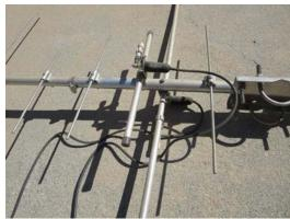
This antenna, still being produced by Cushcraft that retails for \$210 new offers a combined VHF/UHF antenna in one package. Both the VHF and UHF sections individually feature 5 element Yagis for each band. The T-coupler shown can be connected to a transceiver that outputs both a VHF and UHF signal on the same antenna port, or, alternately, separate coaxes can be connected to each antenna separately. The antenna is perfect for Field Day operations with an antenna rotator.
