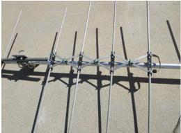
This antenna is an unusual 2-meter antenna in that it has both a Yagi high-gain portion of the antenna combined with a Log Periodic portion of the antenna for wide bandwidth. The antenna is perfect for Field Day operations with an antenna rotator.
