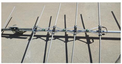
This antenna is an unusual 2-meter antenna in that it has both a Yagi high-gain portion of the antenna combined with a Log Periodic portion of the antenna for wide bandwidth. The antenna is perfect for Field Day operations when used in conjunction with a simple TV-type antenna rotator.
