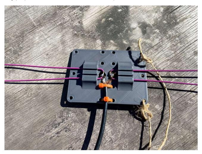
After trimming the longer side to approximately 19" for  $\frac{1}{2}$  wave 2m and the shorter length to approximately 5 7/8" for  $\frac{1}{2}$  wave 70cm, I checked the VSWR using my NanoVNA.
