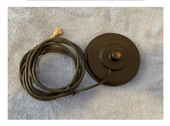
This heavy-duty 5"diameter magnetic antenna mount uses a powerful 2.5 pound magnetic base for secure mounting on top of most vehicles. It features a standard 3/8-24 threaded receptacle for attaching various hamstick or other whip antennas as needed. The 9-1/2 ft. length of RG-58 cable has a standard PL-259 UHF end connector. Typical cost of this magnetic antenna mount from MFJ or DX Engineering is \$29.95.
