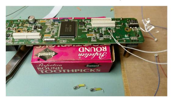
Put the control board back on, plugged it in, and measured the voltage. The actual LCD is still removed. 10.7 volts is fine, I will just pick a resistor to match that voltage. 1 K Ohm resistor will give 10 milli-Amps through the LED, well under its capability with no heat sink.
