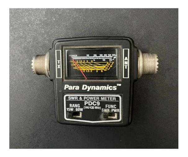
The Para Dynamics PDC9 inline SWR / Power Meter operates from 144MHz to 430MHz which includes the 2m - 70cm ham bands. The unit has two power ranges, 15W and 60W. Unit provides two female SO-239 coax connectors. Unit measures approximately 2" X 2.5" X 1". A similar unit recently sold on eHam.net for \$25.
