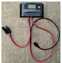
I used 10 gauge red/black wire to connect the solar panel to the charge controller and from the charge controller to the battery box. I terminated the solar panel side with MC4 connectors and the battery side with 45 amp Anderson powerpole connectors. The connectors were all crimped and soldered.
