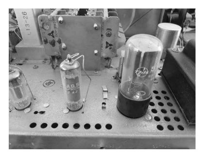
And on the bottom of the audio amplifier tube is a resistor and capacitor (the lighter grey tube with the blue symbols).
