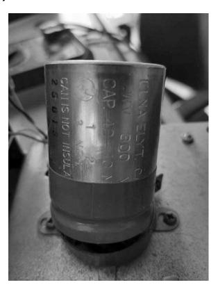
The multi section cap is right near the input transformer and rectifier tube that turns AC input DC (the fat one on the right). The skinny tube in the middle (with the wire clip) is the final audio amplifier tube.
