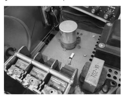
Yup, 40 uF at 300 volts, just like the schematic.
