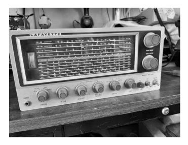
What makes radios that were built in **1965** hum? There are only a few types of components in this radio - tubes, resistors, transformers, and capacitors. Since the receiver works, and the hum is on all bands, this problem maybe comes from a capacitor not filtering out the rectified AC power. Aluminum electrolytic capacitors have a finite life span and so is the mostly likely suspect. 60 years is probably way past the expected life.
