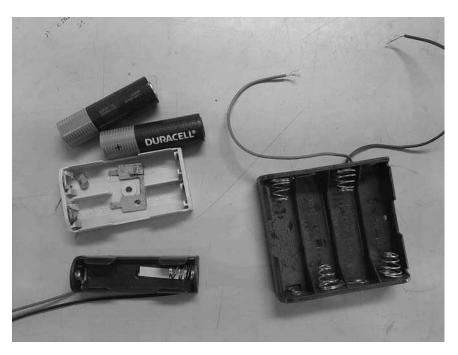
Rather than resorting to buying something new, I have an option already sitting around. An AA battery has 2,000 to 2,500 mAh capacity. I have a pouch LIPO cell with 5,000 mAh capacity. **How about putting it underneath the card stock**? Probably could power my tinkering for 6 months as often as I play with this. A bit of velcro, connect the wires to the bottom side of the spring connectors, and it is **ready to go**.
