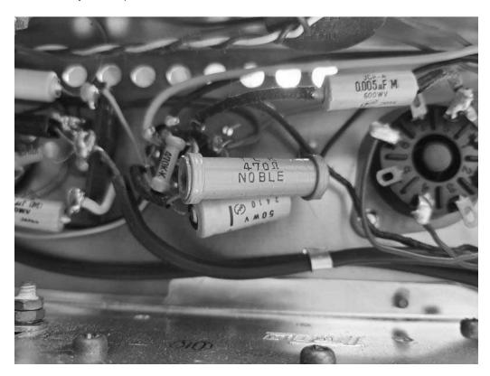
Just to check, I used a voltmeter to check things out. 1st, I made sure this older radio did not have a "hot" chassis, that **could shock you** depending on which way you plugged in the line cord. **Both plug tabs are the same size, and no ground pin**.
